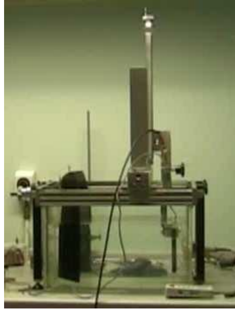
Figure 3.1: Experimental set-up for the beam-profiling showing the water tank with the positioning gantry over the top holding the membrane hydrophone. The Doppler probe can just be seen inserted in the Right-hand end of the tank.
