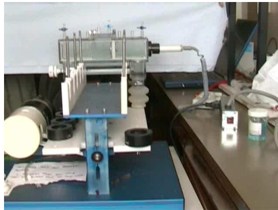
Figure 4.1: The Shelhigh Accelerated Rate Fatigue tester showing the set-up used for this project
