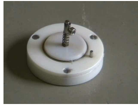
Figure 4.3: A simple spring-loaded valve
