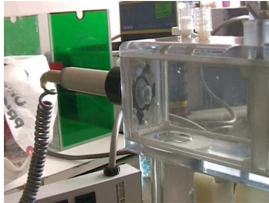
Figure 4.2: The Doppler probe held in place at one end of the Shelhigh Wear tester
